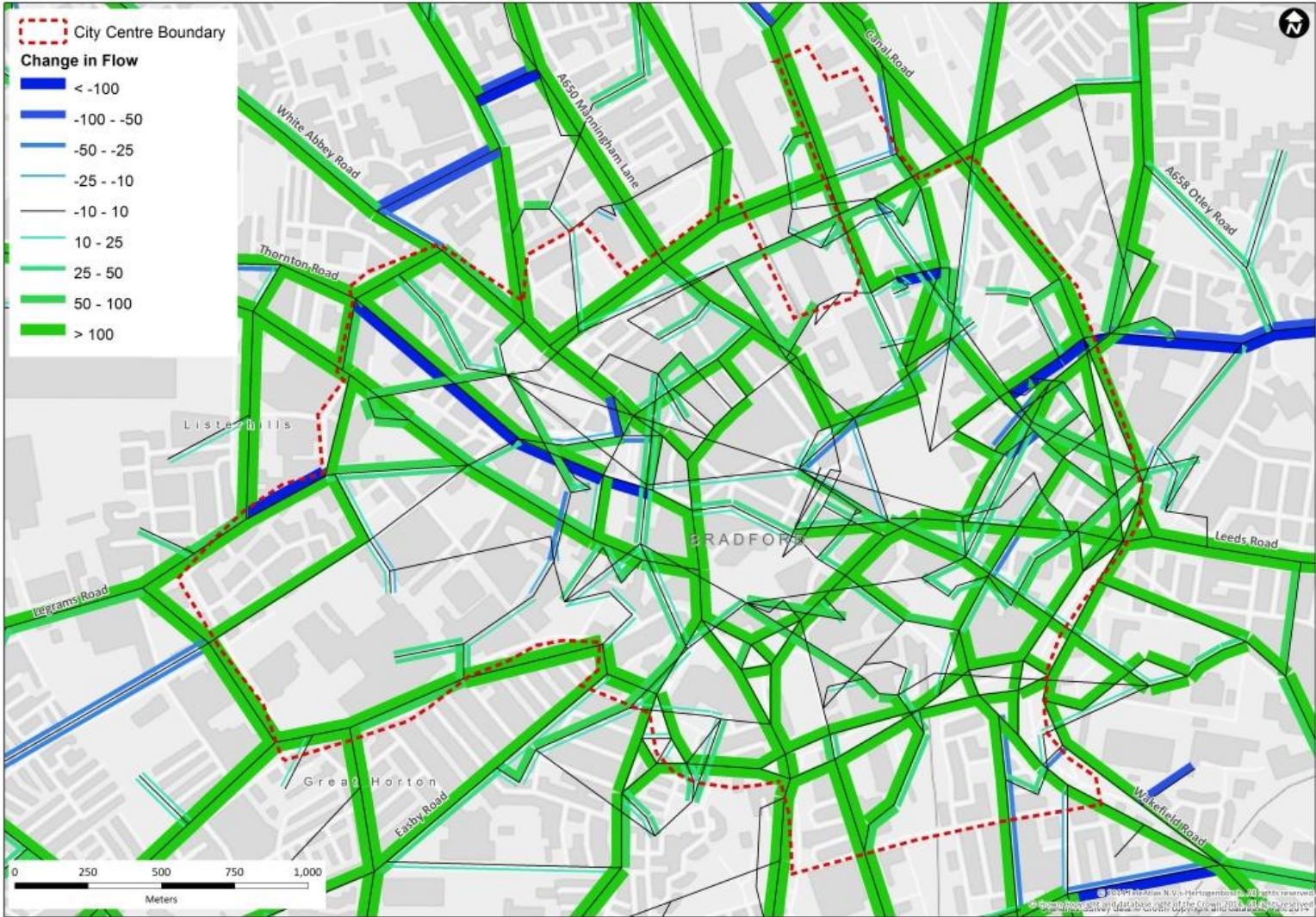
Figure A.2: Difference in flow – 2030Forecast year minus Base Year – AM peak hour
