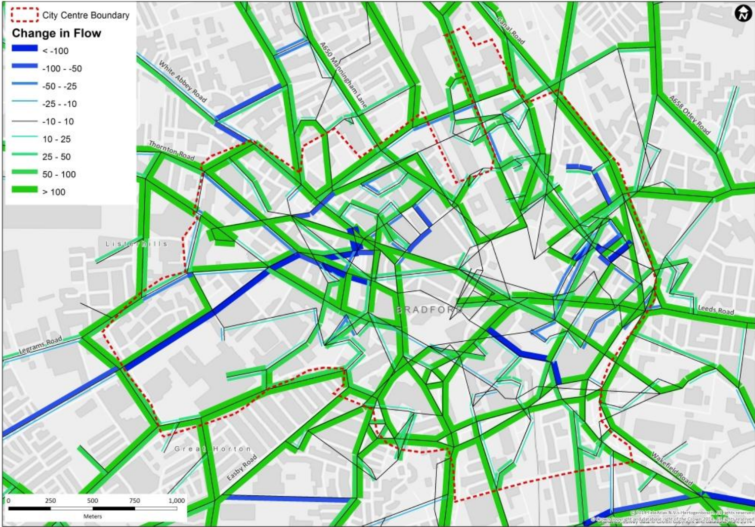
Figure A.3: Differences in flow – 2030 Forecast Yea minus Base Year – PM peak hour
